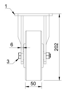
UNLESS OTHERWISE **SPECIFIED** DIMENSIONS ARE IN **MILLIMETRES**
