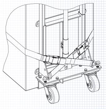
Straps cross over at rear of load, hooked to the eyebolts with cam buckles behind the Skoots frames
