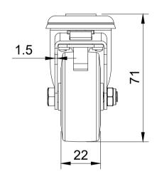
**Unspecified Tolerances** Machining ± 0.25mm Fabrication ± 1mm
