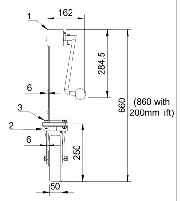
UNLESS OTHERWISE SPECIFIED DIMENSIONS ARE IN MILLIMETRES
