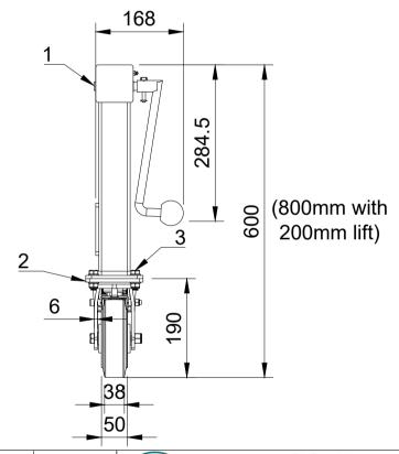
UNLESS OTHERWISE SPECIFIED DIMENSIONS ARE IN MILLIMETRES
