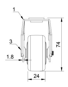
UNLESS OTHERWISE **SPECIFIED** DIMENSIONS ARE IN MILLIMETRES
