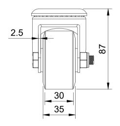
Unspecified Tolerances Machining ± 0.25mm Fabrication ± 1mm
