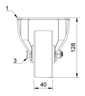
UNLESS OTHERWISE **SPECIFIED** DIMENSIONS ARE IN **MILLIMETRES**
