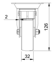
UNLESS OTHERWISE SPECIFIED DIMENSIONS ARE IN MILLIMETRES
