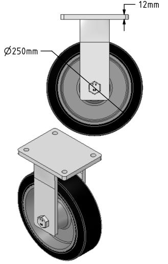
Fabricated fixed castor with a flat plate fixing fitted with a black elastic rubber tyred cast iron centred wheel with ball bearing. Wheel diameter 250mm, tread width 75mm, overall height 314mm, plate size 175mm x 140mm, hole centres 140mm x 105mm.
