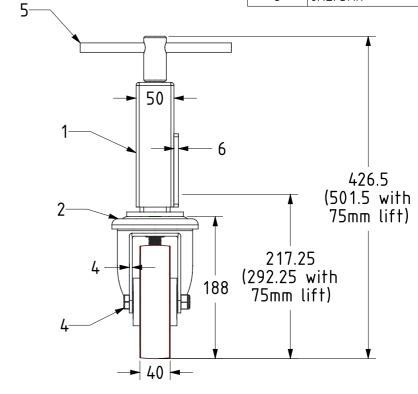
UNLESS OTHERWISE SPECIFIED DIMENSIONS ARE IN MILLIMETRES
