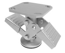
Pressed Steel Construction with a mounting height of 195mm. Retracted height 155mm. Plate size 115mm x 102mm with hole centres of 82/76mm x 67/76mm. Truck locks are NOT designed to carry any weight and are used as a form of brake.
