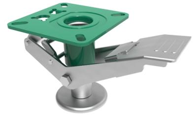
BZTL6 is a roll lock which is comprised of a pressed steel construction, with rubber foot pads of 80mm diameter. Mounting height 210mm, with retracted height of 170mm, 120mm x 120mm top plate, 100mm X 100mm OR 85mm x 85mm bolt holes.
