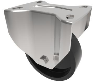
Pressed steel fixed castor with a top plate fixing fitted with a black thermoplastic wheel with PTFE bushes. Wheel diameter 100mm, tread width 30mm, overall height 128mm, top plate 105mm x 80mm, hole centres 80mm x 60mm or 75mm x 45mm. Load capacity 200kg at 280c consent and 280c peak temperature..REACH compliant, RoHs Compliant, USDA approved FDA approved.
