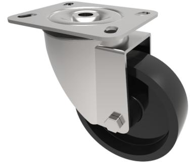
Pressed steel swivel castor with a top plate fixing fitted with a black thermoplastic wheel with PTFE bushes. Wheel diameter 100mm, tread width 30mm, overall height 128mm, top plate 105mm x 80mm, hole centres 80mm x 60mm or 75mm x 45mm. Load capacity 200kg at 280c consent and 300c peak temperature. REACH compliant, RoHs Compliant, USDA approved FDA approved.
