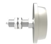
Flanged steel radiused wheel with ball bearings and steel axle. Wheel diameter 55mm, outer flange 70mm, tread width 25mm, hub length 35mm. Axle M16, Load capacity 160kg. Suitable for use with ( RSC ) Rolled steel channels.
