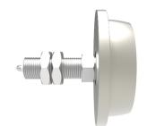
Flanged steel radiused wheel with ball bearings and steel axle. Wheel diameter 175mm, outer flange 200mm, tread width 35mm, hub length 50mm. Axle M36, Load capacity 1500kg. Suitable for use with ( RSC ) Rolled steel channels.
