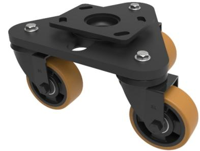
Central heavy duty black painted swivel head mounted on a black painted triangular base plate fitted with 3 pressed steel black painted swivel castors fitted with brown polyurethane tyred black nylon centred wheels with roller bearings. Wheel diameter 125mm, tread width 45mm, overall height 192mm. Load capacity 600kg.
