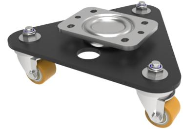
Central medium duty swivel head, mounted on a triangular base plate fitted with 3 pressed steel swivel castors fitted with 35mm brown 92 shore A polyurethane tyre steel centred wheels with ball bearings. Overall height 84mm, Mounting Plate size 115 x 85mm, hole centres 80 x 60mm, Load capacity 225kg.
