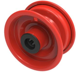
Welded 1.8mm gauge steel rim to suit 4.00 x 8 tyres with a 25mm x 65mm bore red powder coated finish Max inflated on this rim is 36 psi
