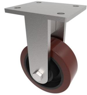
**POA** Fabricated fixed castor with a flat plate fixing fitted with a brown polyurethane tyre on cast iron centred wheel with ball bearings. Wheel diameter 400mm, tread width 125mm, overall height 552mm, plate size 178mm x 153mm, hole centres 127mm x 102mm. Load capacity 4600kg. **\*\*MANUFACTURED TO ORDER\*\***
