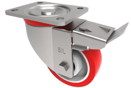
Pressed steel swivel castor with a top plate fixing fitted with a red polyurethane tyre on white nylon centred ball bearing wheel and total lock brake. Wheel diameter 125mm, tread width 40mm, overall height 164mm, plate size 135mm x 110mm, hole centres 105mm x 80mm. Load capacity 300kg. NB due to the fact these are reinforced nylon the white centre is slightly off white.
