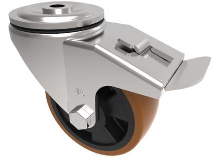
Pressed steel swivel castor with a 12mm bolt hole fitted with a brown polyurethane tyre on black nylon centred wheel with a roller bearing and total lock brake. Wheel diameter 100mm, tread width 40mm, overall height 128mm, Load capacity 300kg
