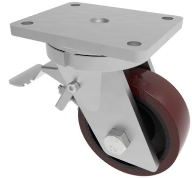
Fabricated swivel castor with a top plate fixing fitted with a polyurethane tyred cast iron centred wheel with ball bearings and total lock brake. Wheel diameter 150mm, tread width 50mm, overall height 212mm, top plate 175mm x 140mm, hole centres 140mm x 105mm. Load capacity 750kg.
