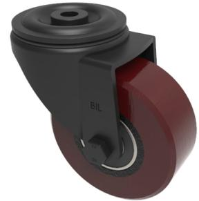
Pressed steel black painted swivel castor with a 12mm bolt hole fitted with a brown polyurethane tyred cast iron centred wheel with ball bearings. Wheel diameter 100mm, tread width 30mm, overall height 128mm, Load capacity 250kg. ( Catalogue SKU BLKH100PTBJH12)
