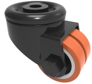
Pressed steel swivel black painted castor with a 12mm bolt hole fitted with 2 x brown polyurethane tyred cast iron centred wheel with plain bore. Wheel diameter 50mm, tread width 2 x 14mm, overall height 73mm, Load capacity 160kg.
