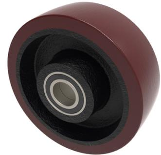
Brown polyurethane wheel on a cast iron centre with ball journal bearings. Wheel diameter 150mm, tread width 50mm, bore 25.4mm, hub 60mm. Load capacity 750kg. NB with this wheel we would take a standard wheel with a 47mm x 14mm bearing seat and fit a 6005 ball bearing but this will set the bearings back in to the wheel hub 2mm each side..
