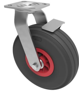
Fabricated swivel castor with a top plate fixing fitted with a 4 ply black ribbed pattern pneumatic tyre with a red polypropylene centre with plain bore and side fitting wheel brake. Wheel diameter 260, tread width 85mm, overall height 318mm, plate size 115mm x 105mm, hole centres 92mm x 67 or 76mm x 76mm. Load capacity 120kg. at max speed 4KPH, for non-towing applications please note we manufacture to order and therefore a 24 hour delivery may not be possible.
