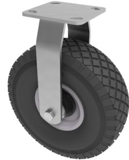
Fabricated fixed castor with a top plate fixing fitted with a 4 ply black diamond pattern pneumatic tyre with a steel disc centre with roller bearings. Wheel diameter 400, tread width 100mm, overall height 480mm, plate size 150mm x 150mm, hole centres 105mm x 80mm. Load capacity 300kg.at max speed 4KPH, for non-towing applications please note we manufacture to order and therefore a 24 hour delivery may not be possible.
