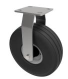
Fabricated fixed castor with a top plate fixing fitted with a 4 ply black ribbed pattern pneumatic tyre with a grey steel centre and roller bearing. Wheel diameter 260, tread width 85mm, overall height 318mm, plate size 115mm x 105mm, hole centres 92mm x 67 or 76mm x 76mm. Load capacity 200kg.at max speed 4KPH, for non-towing applications please note we manufacture to order and therefore a 24 hour delivery may not be possible..
