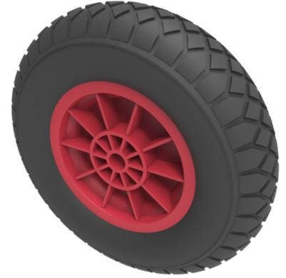
Black pneumatic tyre on red polypropylene centre rim with a plain bore. Fitted with a 4 ply diamond tread patterned tyre. Wheel diameter 400mm, tread width 100mm, hub 66mm, bore 25.4mm. Load capacity 200kg at 4KPH, for non-towing applications please note we manufacture to order and therefore a 24 hour delivery may not be possible. Important notice : Refer to rim ing not the tyre
