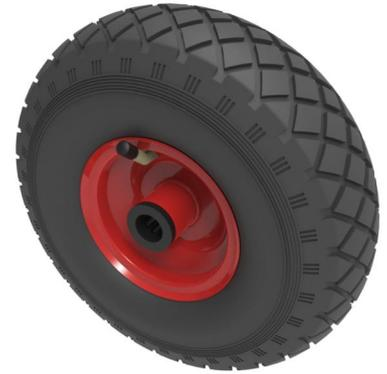
Black pneumatic tyre on red steel centre rim with a roller bearing. Fitted with a 4 ply diamond tread patterned tyre. Wheel diameter 260mm, tread width 85mm, hub width 75mm, bore 20mm. Load capacity 200kg at 4KPH, REACH COMPLIANT. Not recommended for foam filling please take advise from the BIL Technical department or consider the BIL puncture proof range. for non-towing applications please note we manufacture to order and therefore a 24 hour delivery may not be possible.
