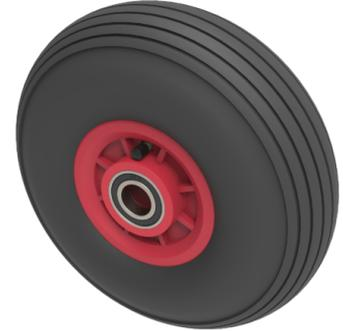
Black pneumatic tyre on red polypropylene centre rim with a ball bearings. Fitted with a 4 ply ribbed tread patterned tyre. Wheel diameter 260mm, tread width 85mm, hub 75mm, bore 25mm. Load capacity 120kg at 4KPH, for non-towing applications please note we manufacture to order and therefore a 24 hour delivery may not be possible. Important notice : Refer to rim for PSI rating not the tyre
