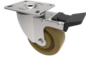
Stainless steel grade 304 swivel castor with a top plate fixing fitted with a brown phenolic wheel with a plain bore with total lock brake. Wheel diameter 100mm, tread width 38mm, overall height 128mm, top plate 100mm x 85mm, hole centres 80mm x 60mm or 75mm x 45mm. Load capacity 150kg at a maximum temperature of 250c.
