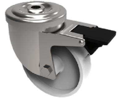
Grade 304 Stainless steel swivel castor with a 12mm bolt hole fixing fitted with a off white nylon wheel with a plain bore and a total lock brake. Wheel diameter 80mm, tread width 36mm, overall height 110mm. Load capacity 190kg at 130c maximum temperature. **\*\*MANUFACTURED TO ORDER\*\***
