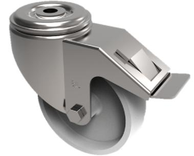
Grade 304 Pressed stainless steel swivel castor with a 12mm bolt hole fitted with a white nylon wheel with a roller bearing and a total lock brake. Wheel diameter 100mm, tread width 32mm, overall height 130mm, Load capacity 250kg
