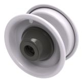
Rim steel 4.00 X 8 with a 20MM X 75MM bore grey powder coated finish Max inflated on this rim is 36 psi
