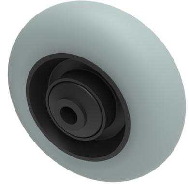
Grey 55 shore A round profile elastic rubber tyre on black nylon centred wheel with a single ball bearing with retaining caps. Diameter 125mm, tread width 38mm, bore size 10mm, hub length 47mm. Load capacity 170kg. REACH compliant also PAH-Free rubber to confirm to EU-directive 2005/69/EC
