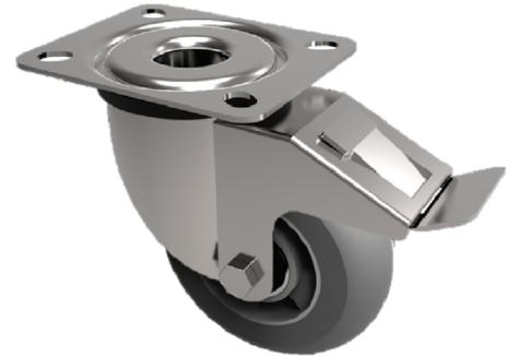
Grade 304 Pressed stainless steel swivel castor with a top plate fixing fitted with a grey high elastic natural 55 shore A round profile rubber tyre aluminium centred wheel with stainless steel ball bearings. Wheel diameter 125mm, tread width 40mm, overall height 155mm, top plate 105 x 85mm, hole centres 80mm x 60mm. Load capacity 200kg. REACH compliant also PAH-Free rubber to confirm to EU-directive 2005/69/EC,
