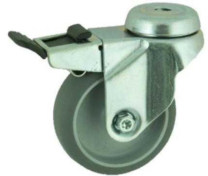
Grade 304 Pressed stainless steel swivel castor with a 10mm bolt hole fitted with a grey thermoplastic rubber tyre on polypropylene centred wheel with a plain bore and a total lock brake. Wheel diameter 100mm, tread width 24mm, overall height 124mm. Load capacity 70kg
