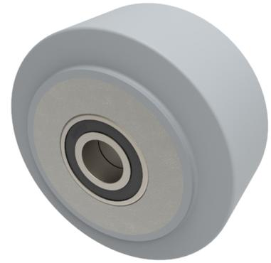
Grey high elastic natural 65 shore A rubber tyre on aluminium centred wheel with ball bearings. Diameter 80mm, tread width 40mm, bore size 15mm, hub length 40mm. Load capacity 180kg. REACH compliant also PAH-Free rubber to confirm to EU-directive 2005/69/EC. REACH compliant also PAH-Free rubber to confirm to EU-directive 2005/69/EC
