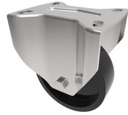
Pressed stainless steel fixed castor with a top plate fixing fitted with a 280C grey technopolymer reinforced with glass fiber wheel with a plain bore and a stainless steel axle tube. Wheel diameter 100mm, tread width 32mm, overall height 128mm, top plate 105mm x 85mm, hole centres 80mm x 60mm Load capacity 180kg. (BIL always recomend using a PTFE bush in case of wheel scream)
