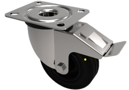
Grade 304 stainless steel swivel castor with a top plate fixing fitted with a 65 shore A black elastic electrically conductive rubber wheel on a black nylon centre with a ball bearing (NB the ball bearing is not stainless steel) and a total lock brake. Wheel diameter 80mm, tread width 35mm, overall height 105mm, top plate 105mm x 85mm, hole centres 80mm x 60mm Load capacity 100kg. Conductivity range is  $10^3$  ohm to  $10^4$  ohm
