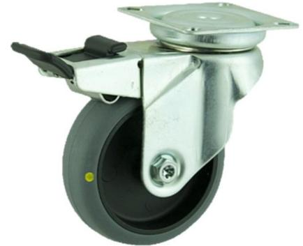
Grade 304 Stainless steel swivel castor with a top plate fixing fitted with a grey electrically conductive tyre on a black polypropylene centred wheel with ball bearing and a total lock brake. Wheel diameter 75mm, tread width 32mm, overall height 109mm, top plate 90mm x 70mm, hole centres 75mm x 56mm or 64mm x 44mm. Load capacity 70kg. Conductive offers a resistance  $R < 10 \Omega$  **\*\*MANUFACTURED TO ORDER\*\***
