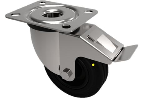
Grade 304 Stainless steel swivel castor with a top plate fixing fitted with a 65 shore A black elastic electrically conductive rubber wheel on a black nylon centre with ball bearings and a total lock brake. Wheel diameter 200mm, tread width 50mm, overall height 235mm, top plate 135mm x 110mm, hole centres 105mm x 80mm Load capacity 350kg. Conductivity range is  $10^3$  ohm to  $10^4$  ohm
