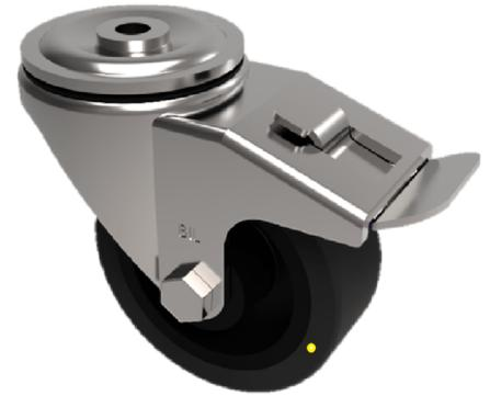
Grade 304 Stainless steel swivel castor with a bolt hole fixing fitted with a 65 shore A black elastic electrically conductive rubber wheel on a black nylon centre with ball bearings (Not stainless steel) with total lock brake. Wheel diameter 125mm, tread width 36mm, overall height 155mm, bolt hole 12mm. Load capacity 200Kg. Conductivity range is  $10^3$  ohm to  $10^4$  ohm
