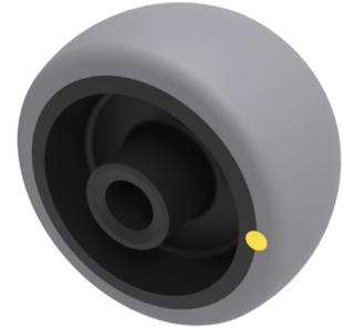
Grey electrical conductive rubber on polypropylene wheel with plain bore. Wheel diameter 50mm, tread width 24mm, Hub width 28mm, Bore size 8mm. Load capacity 50kg Conductive offers a resistance  $R < 10^{10} \Omega$
