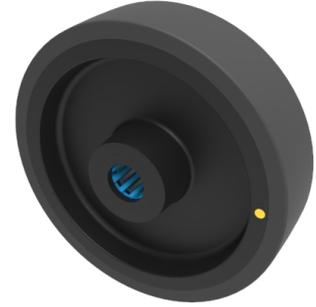
Black electrically conductive polyurethane tyre on black nylon centred with stainless steel roller bearing wheel. Wheel diameter 160mm, tread width 40mm, bore size 20mm, hub length 58mm. Load capacity 320kg Conductive offers a resistance  $R < 10000 \text{ Ohm}$  **\*\*MANUFACTURED TO ORDER\*\***
