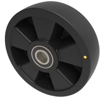
Black electrically conductive nylon wheel with ball bearings. Wheel diameter 200mm, tread width 57mm, Hub width 59mm, Bore size 25mm. Load capacity 520kg Conductive offers a resistance  $R < 10000 \text{ Ohm}$
