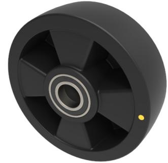
Black electrically conductive nylon wheel with ball bearings. Wheel diameter 160mm, tread width 50mm, Hub width 55mm, Bore size 25.4mm. Load capacity 325kg Conductive offers a resistance  $R < 10000 \text{ Ohm}$
